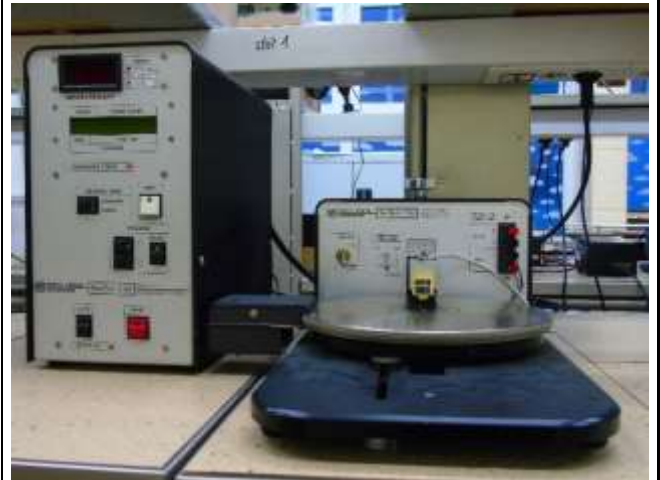
Four-point probe with measuring system for determining surface resistance of silicon diffusion layers
