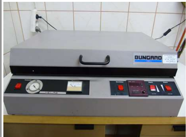
High precision vacuum exposure unit used for selective deposition of thin metallic layers
