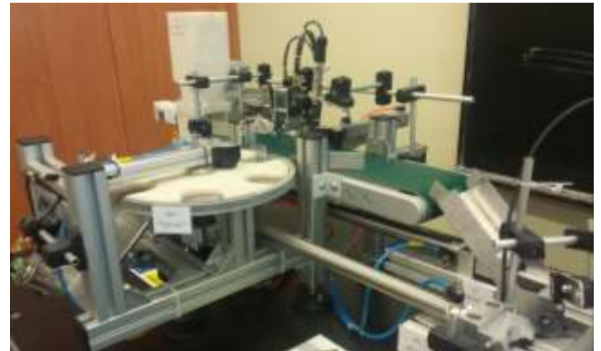
Fig. 2. The input and transport module with carousel warehouse
