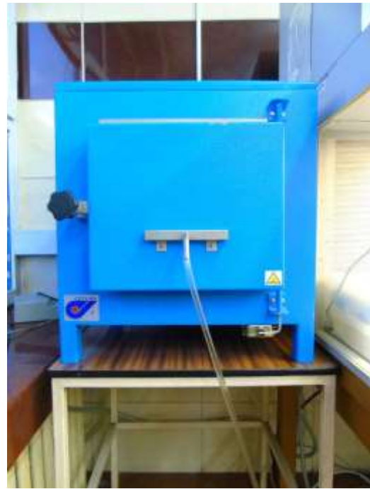
Chamber furnace for heat treatment of spin-on and spray-on glazes
