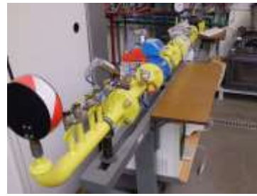
The station for the research of gas meters and gas flow
