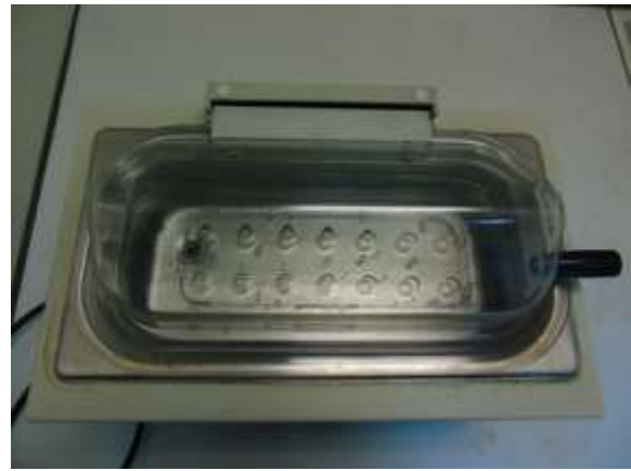
The inside of the chamber for the chemical process of metallization with Ni-P alloys
