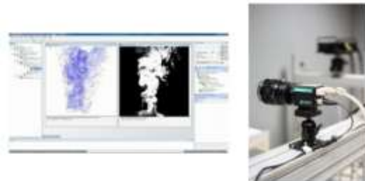
4. Particle Image Velocimetry (PIV) – optical method of flow analysis
