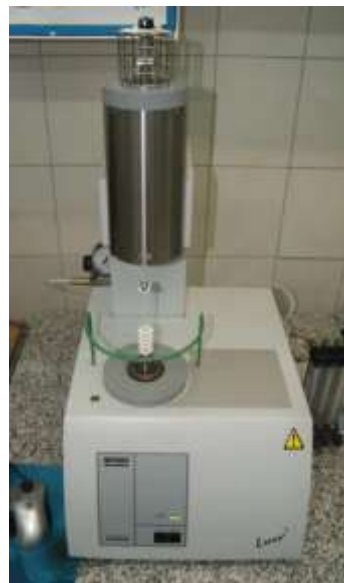
Device STA 409PG/6 for thermal analysis DSC/TG of materials
