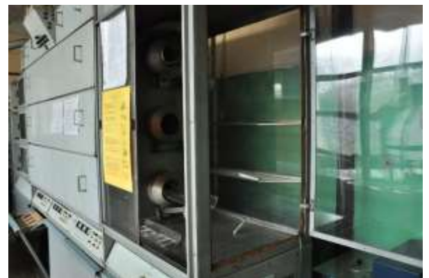
Tunnel Furnace for heating and oxidation of thin sensory layers
